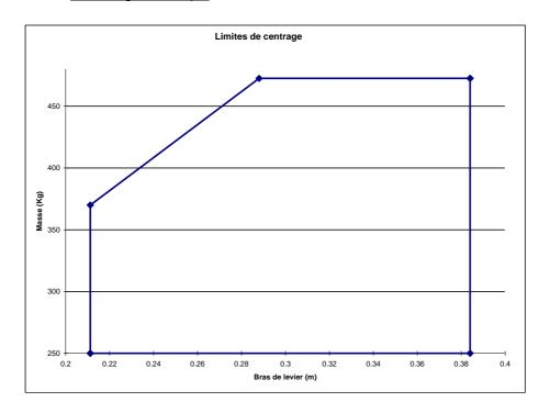
M.A.C. =960 mm; Reference datum: 13.5 mm ahead of left wing leading-edge.
